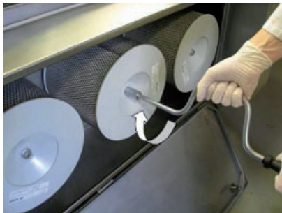
Sealing mechanism from the outside (non-contaminated).
